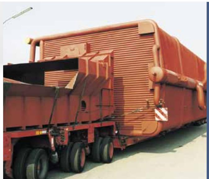
Figure 2: 100 MW hot water - water tube boiler during transport
