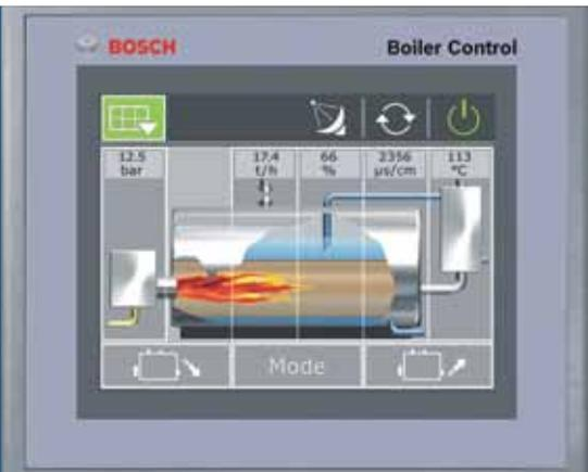
Touch-screen display on the BOILER CONTROL BCO on a steam boiler with Economiser
