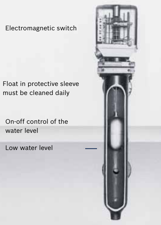
Figure 1: Float-type water level limiter – checking the safety circuit and daily blow-through cleaning are obligatory
