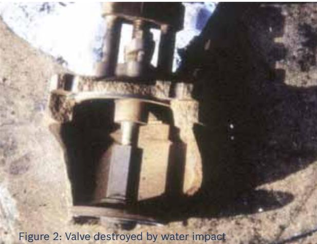
Figure 2: Valve destroyed by water impact
